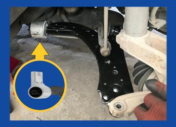
Apply sufficient force to push the wishbone bush into the location hole. This will allign the bushes and the ball joint for fitment.
