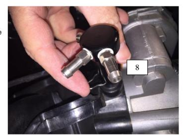
9. Once installed, the boost reference adapter should look as shown. Vacuum hoses can now be connected.
