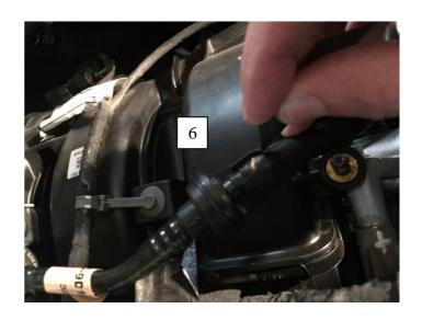
Slide the boost reference adapter onto the OEM port as shown. Twist adapter back and forth while pressing down as there will be some resistance due to the internal O-ring.
