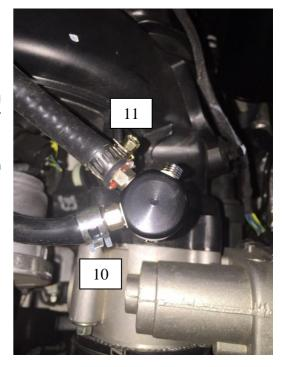
12. Install other end of ½" re-inforced hose over barbed end of PCV check valve as shown. No clamp is needed.
