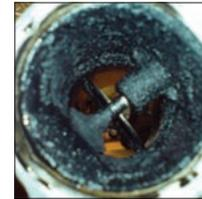
EGR valve which is malfunctioning due to excessive carbon / coke.
